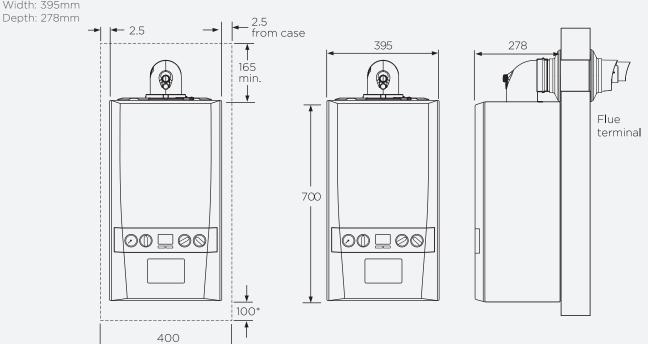
Note: The minimum front clearance when built in to a cupboard is 5mm from the cupboard door but 450mm overall clearance with the cupboard door open is required for servicing. \*Bottom clearance after installation can be reduced to 5mm. However, 100mm is required for servicing.
