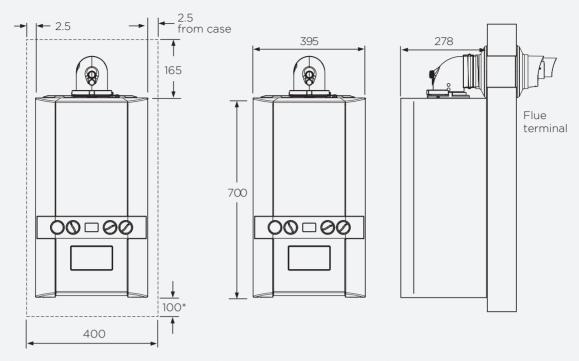
Note: The minimum front clearance when built-in to a cupboard is 5mm from the cupboard door but 450mm overall clearance with the cupboard door open is required for servicing. \*Bottom clearance after installation can be reduced to 5mm. However, 100mm is required for servicing.
