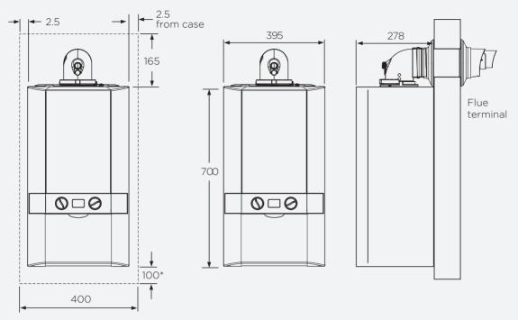
Note: The minimum front clearance when built-in to a cupboard is 5mm from the cupboard door but 450mm overall clearance with the cupboard door open is required for servicing. \*Bottom clearance after installation can be reduced to 5mm. However, 100mm is required for servicing.
